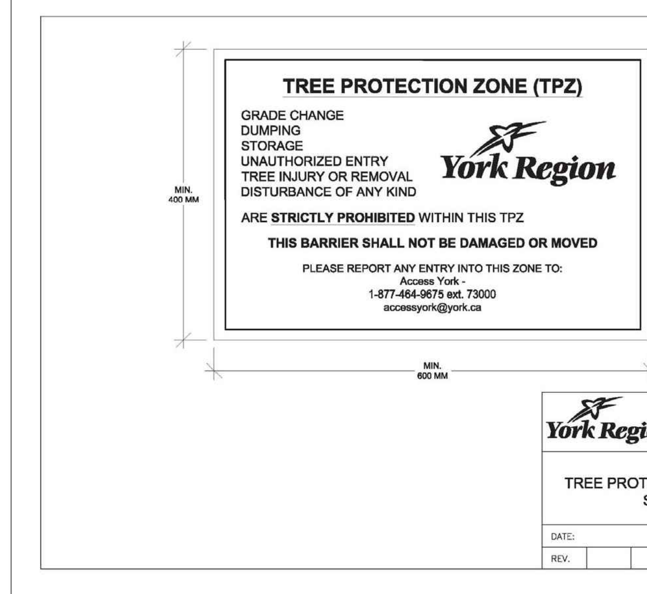
NHF-401: Tree Protection Zone (TPZ) signage
