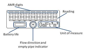
**AMR Digit Bar** (4 to 8 Digits): The AMR digit bar shows which digits will be reported when the meter is read through the communications interface.
