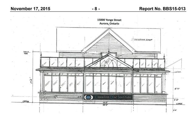
Front Elevation Showing size and location of proposed wall sign
