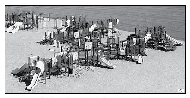
This playspace has more than 20 play components and provides ramp access to elevated play components. The ramp system, consisting of ramp runs and landings, must connect at least 25 percent of the elevated play components. The balance of the elevated components required to be on an accessible route may be connected by the ramp system, or by a transfer system.
