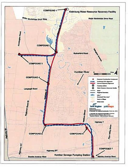
Humber Sewage Pumping Station has been revised to avoid potential issues with respect to existing and future bridge crossings. The alignment was originally planned to travel along Legion Road and is now proposed to follow a City of Vaughan right-of-way, just west of Wallace Street. The proposed modifications will reduce potential disruptions to the community and minimize potential impacts to the natural environment.
