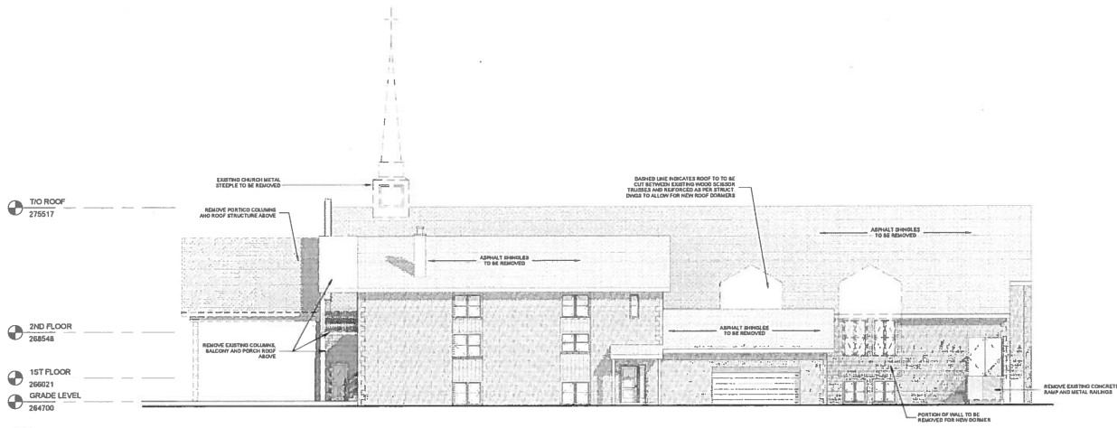
1 SOUTH ELEVATION - DEMOLITION A1.23 1:100
