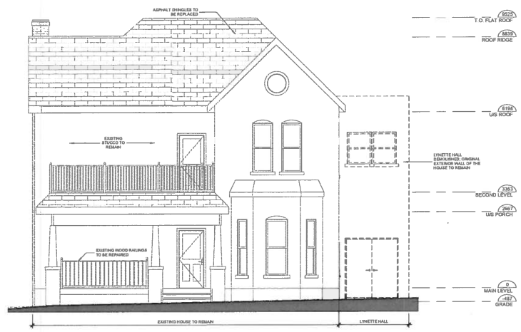
1 A2.21 EXISTING SOUTH ELEVATION 1: 50
