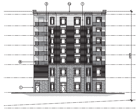
2 NORTH ELEVATION - WEST TOWER SCALE: 1:150
