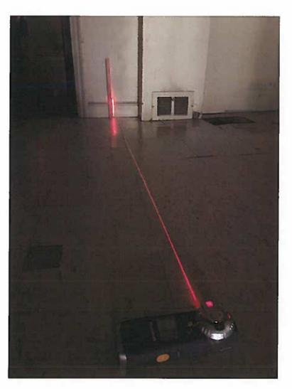
Laser level showing displacement in kitchen floor
