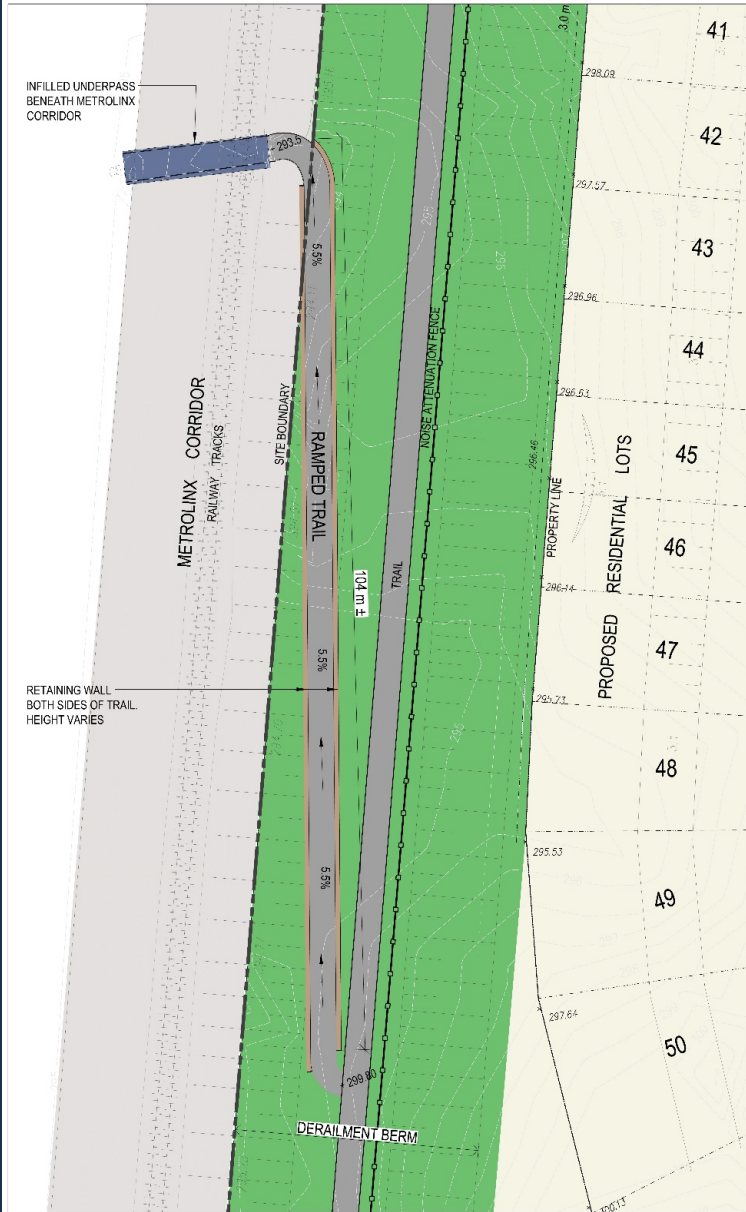
Option A – Ramped Trail with Retaining Walls
