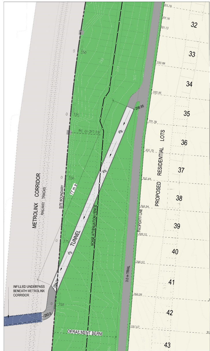
Option B – Angled Concrete Tunnel Through Berm
