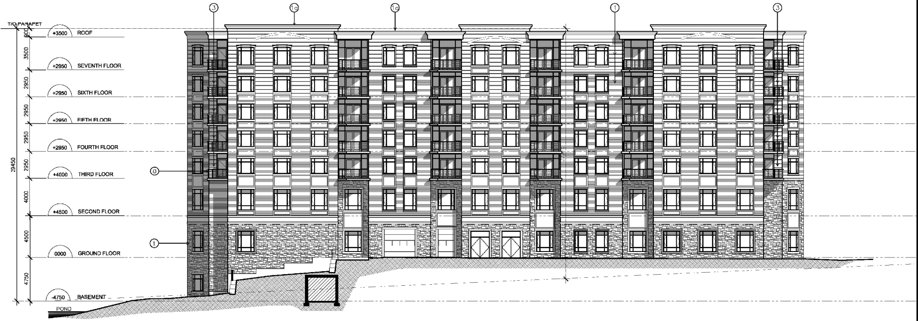
1 EAST ELEVATION - EAST TOWER A-3.3 SCALE: 1:150
