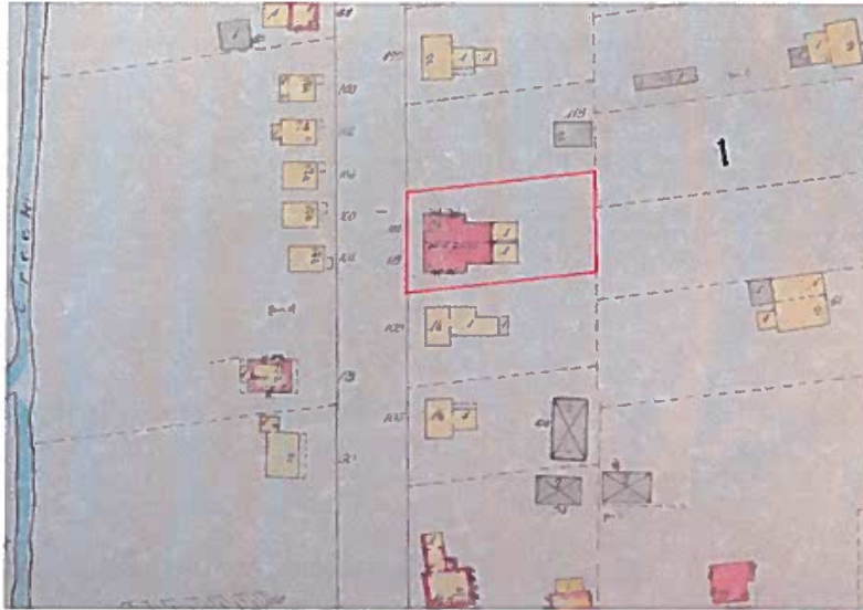
Fire Insurance Map, Town of Aurora, showing the subject property as 2½ storey main structures with 1 storey addition at rear, the main structure is framed with brick veneer. Surveyed March 1904, Revised to November 1913 by Chas E. Goad Co., Civil Engineers. Source: Aurora Historical Society.
