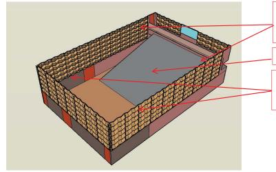
For performances that require the longest reverberation times the side variable drapery would be fully retracted to reveal diffusive finish. For more intimate performances some variable drapery may be deployed.
