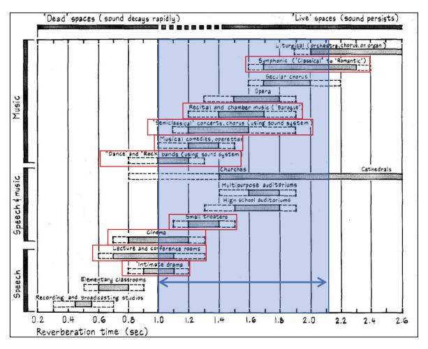
Figure 1. Variable reverberation time within the Multi-Purpose Room
