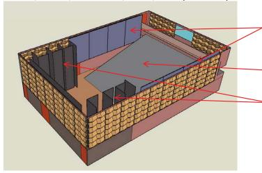
Side variable drapes deployed to control lateral reflections and reduce reverberation within the space. For some uses (musical theatre) the variable drapes may be partially deployed. Wall that are exposed would show diffusive panelling that helps scatter sound and prevents flutter echoes.
