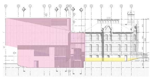
Proposed west elevation, showing new construction in pink, change in grade and foundation to be exposed in yellow (RAW, 2019; Annotated by ERA, 2019).
