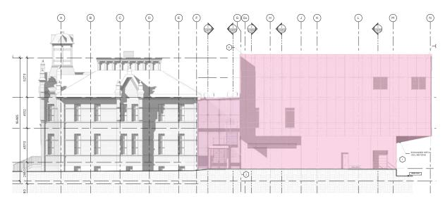
Proposed east elevation, showing new construction in pink (RAW, 2019; Annotated by ERA, 2019).
