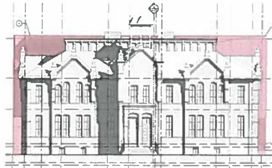
Proposed south elevation, showing new construction behind the heritage building in pink (RAW, 2019; Annotated by ERA, 2019).
